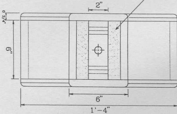
NOTES: 2'-6" height dimension yields a lathe with a center height 44" which is optimum for one Ernie Conover. Elbow point is optimum center height for most turners. Vary 2'-6" height to suit your needs.
